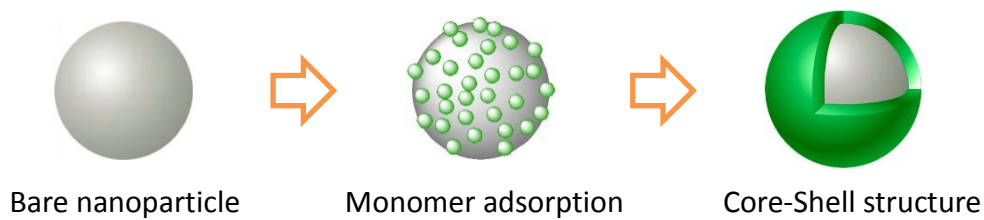
Figure 2.2 – The core-shell structure fabrication process
