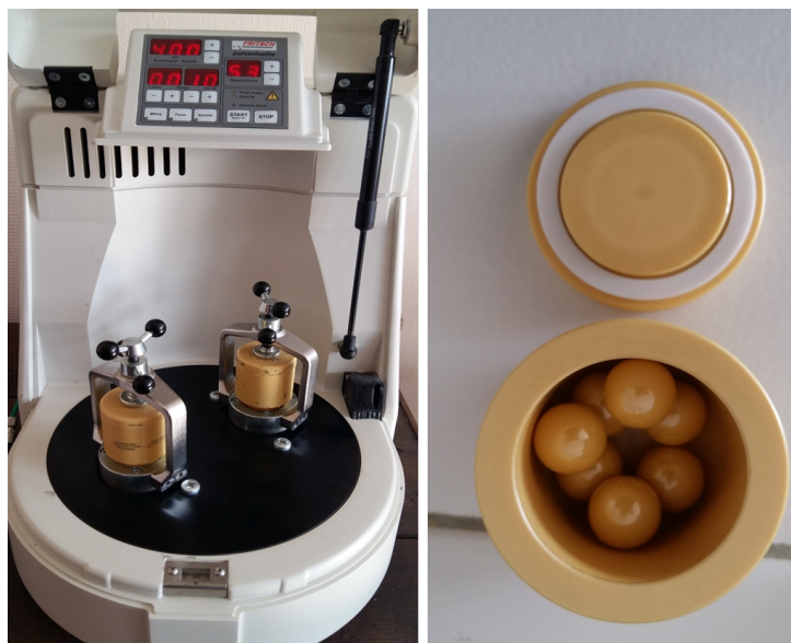
Figure 2.2 – (left) Planetary mill, Pulverisette 7 of Fritsch. (right) Grinding bowl, containing seven balls, used in the planetary ball mill.
