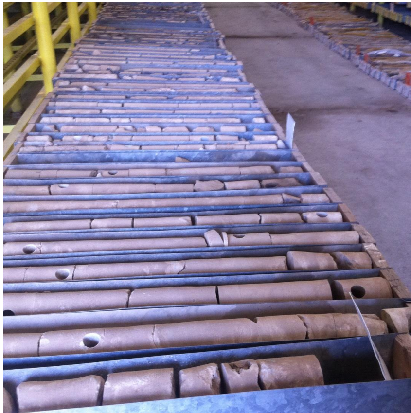
Figure 24 : Example of cores drilled in the Nasiriyah oil field during the collection process of samples
