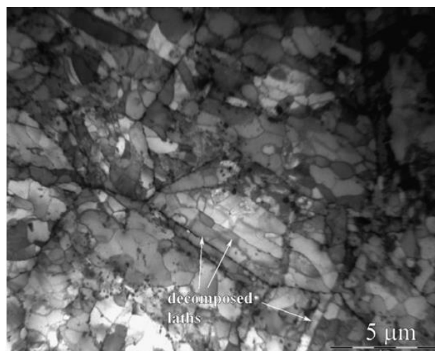
Figure 2-28 Cell structure induced by the cyclic deformation in Eurofer 97 steel, tested at room temperature, at \Delta\epsilon_t=0.8\% , N=7261 cycles [30]
