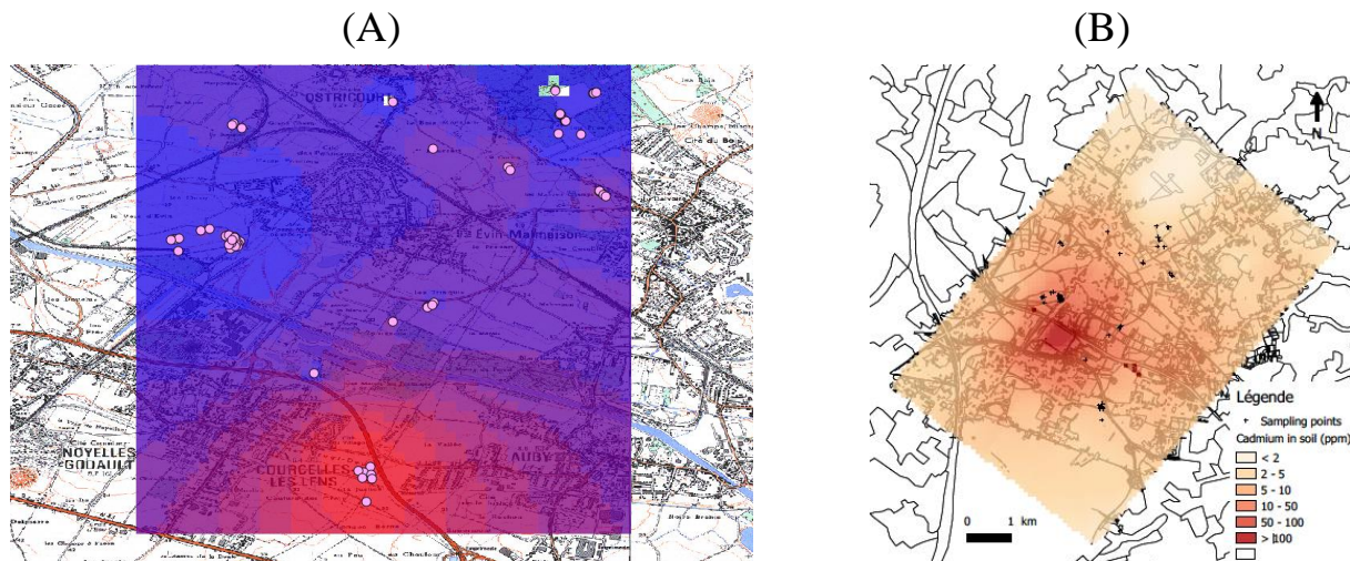
Figure 2 : In A) the distribution of two clusters obtained from samples collected in metals polluted area. The first group is in red in the south and the second one is in blue in the north. In B) cadmium concentration in the soil where samples were collected.
