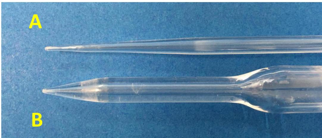
Fig. III.9: The two microprobes tested for GC analysis: A - opening angle of  $10^\circ$  with an orifice diameter of  $300\ \mu\text{m}$ . B- opening angle of  $30^\circ$  with an orifice diameter of  $250\ \mu\text{m}$ .
