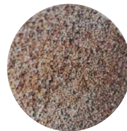
Figure 2. 2. Brick activated with HCl and FeOOH (B+Fe)
