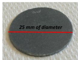
Figure 14 Sample of 25 mm of diameter and 1 mm of thickness for Rheometer test
