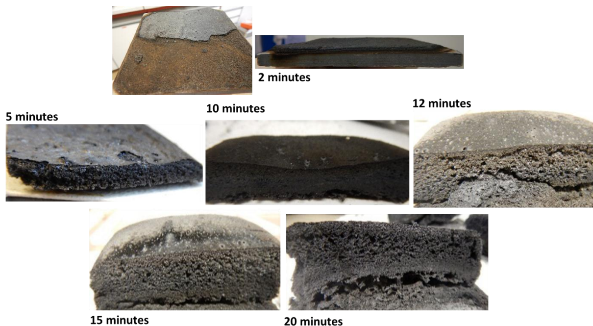
Figure 57 Char appearances of IF(ZB)wt versus times captured by numeric camera
