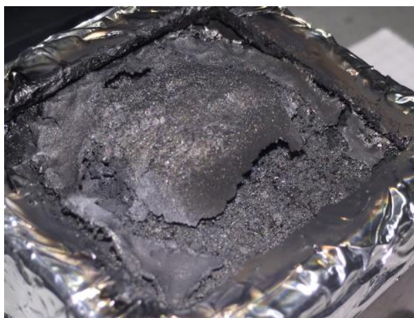
Figure 64: MLC Residual char of PBS/(isosorbide/APP 1/3) 70/30
