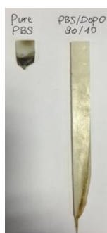
Figure 90: Residual Bars of PBS (left) and PBS/DOPO (right) after the UL-94 testing (3.2 mm).
