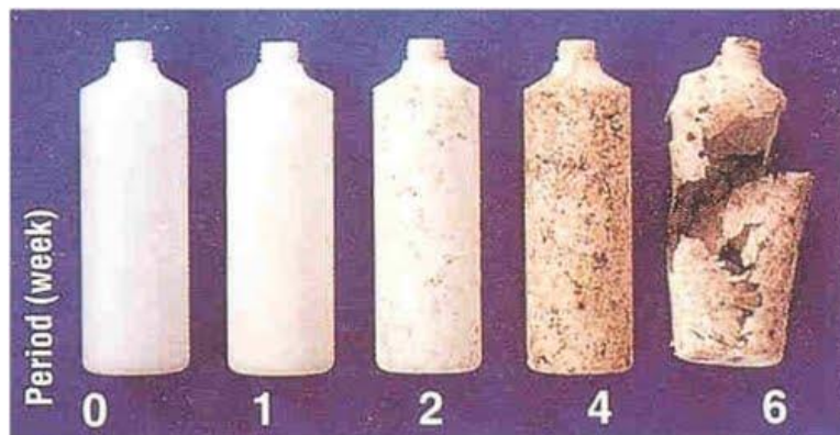
Figure 6: Degradation of PBS in moisture soil
