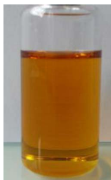
Figure 12. AgNPs coated with amylamine in toluene
