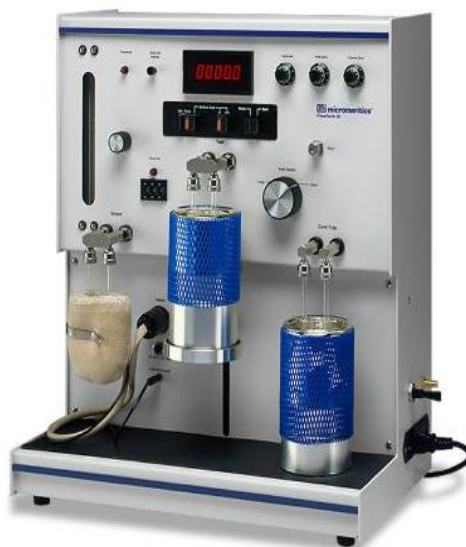
Figure 2.5 – B.E.T. FlowSorb III machine of the laboratory
