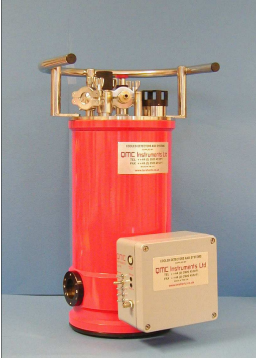
(a) Liquid helium cryostat with a mounted preamplifier
