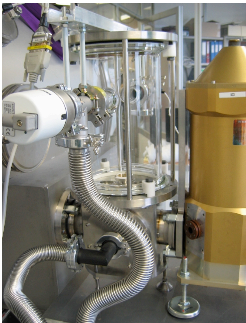
Fig.4: picture of the cell cavity, showing the two pipes for gas injection/removal (front pipe, with gas pressure sensor) and temperature sensor insertion (back pipe). The two golden mirrors of the Offner relay can also be seen on this picture.
