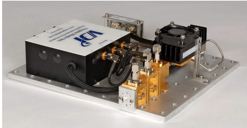
Figure 1.15 – Photograph of a compact AMC from VDI [40].
