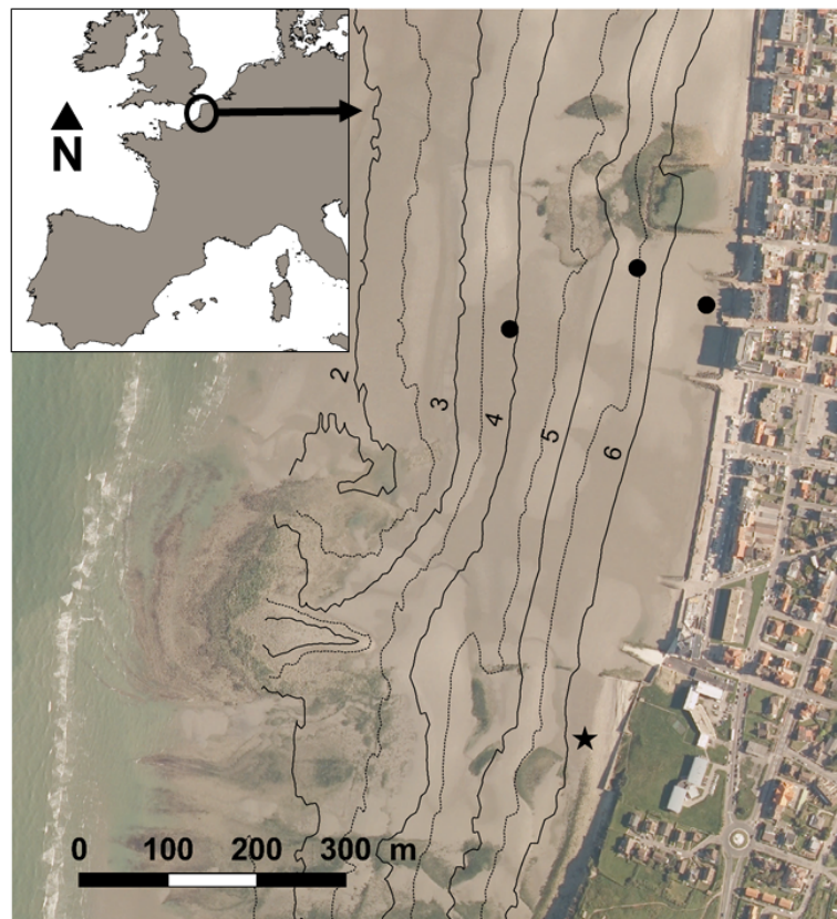
Figure 4.1 – Study site of Wimereux (Eastern English Channel, France) and location of the sampling points for the sediment temperature measurements with two HOBO® Water Temp Pro v2 probes fixed on a metal rod embedded in the sediment (star), and for the size structure of the Arenicola marina population (dots) on different bathymetric levels (lines with numbers) of the foreshore.
