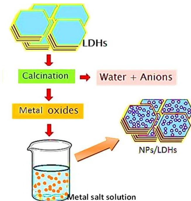
Figure 1.32: The NPs/LDHs nanocomposites synthesis by using the structural memory effect of the layered double hydroxides.
