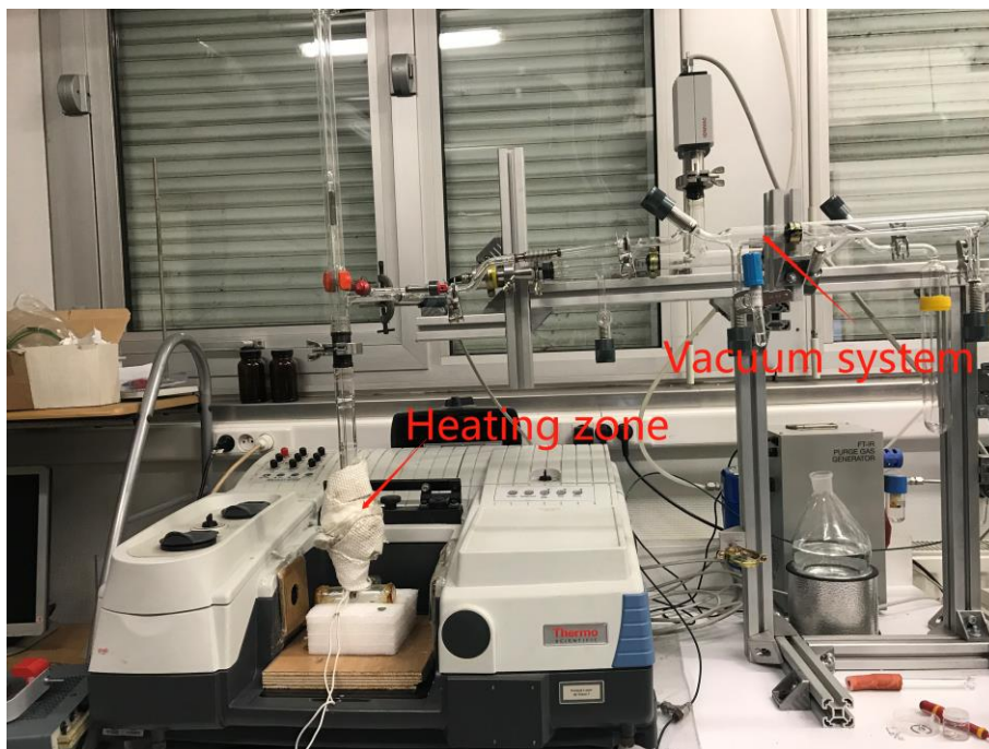
Figure 2.7. Picture of Fourier transform infrared (FT-IR) setup with homemade vacuum system.
