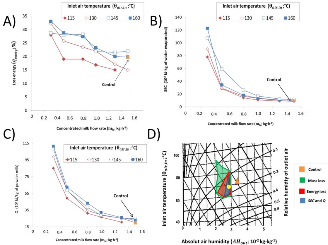
**Figure 4.** Effect of operational parameters on the energetic balance for lactose hydrolyzed milk powder production. A) Energy loss during the LHMP production; B) Energy needed to evaporate 1 kg of water under different drying conditions; C) Energy dispensed to produce 1 kg of LHMP; D) Mollier-Ramzine diagram showing the optimal drying conditions for LHMP production. The yellow point represents LHMP produced with  $\theta_{air,in} = 145$  °C and  $m_{CM} = 1.0$  kg·h<sup>-1</sup>.
