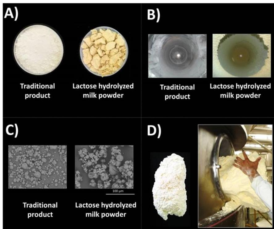
**Figure 4.** Problems associated with production of lactose hydrolyzed milk powder. A) powder browning; B) drying chamber adhesion; C) powder particle agglomeration; D) powder caking.
