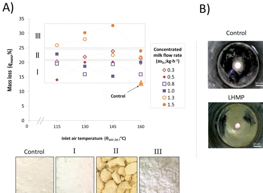
**Figure 3.** Mass loss during the production of lactose hydrolyzed milk powder (LHMP). A) Effect of inlet air temperature and concentrated milk flow rate on the loss mass; B) Images of powder adhesion in the tower drying.
