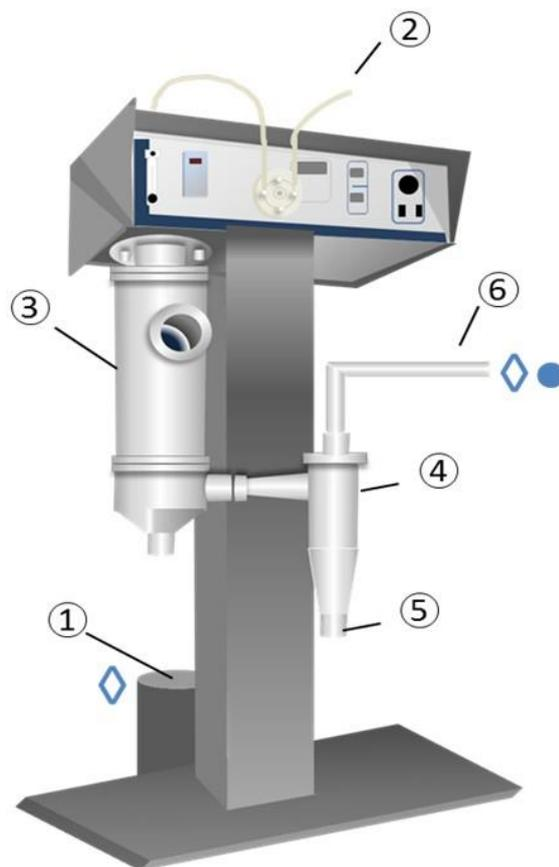
**Figure 2.** Spray dryer diagram. (1) Inlet air; (2) Hydrolyzed lactose concentrated milk pump; (3) drying camera; (4) cyclone; (5) dust collector; (6) outlet air; (◇) position of thermohygrometer; (●) position of anemometer.
