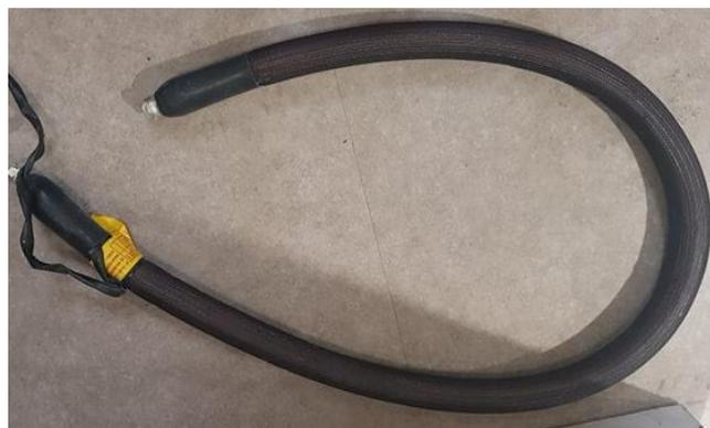
Figure 144. Photo de la gaine chauffante P.E. Heated Hoses Ltd
