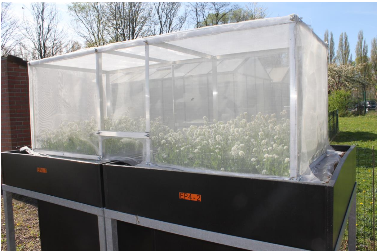
Figure S5 : Insect and wind proof cage system
