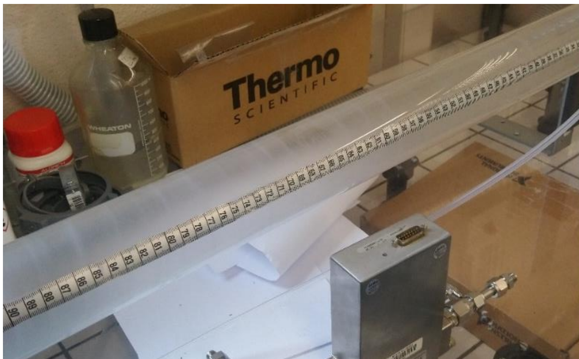
Figure 70: Picture of the AFT whose inner surface has been coated with halocarbon wax.
