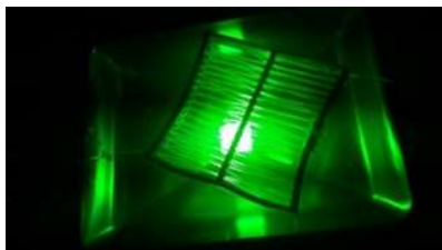
Figure 7-4 - Tubular microreactors: a l = 3.37\text{m} ; i.d. = 800\text{ }\mu\text{m} .
