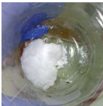
Figure 2-13 \epsilon -PCL obtained from e -ROP in flow by using cholesterol as an initiator
