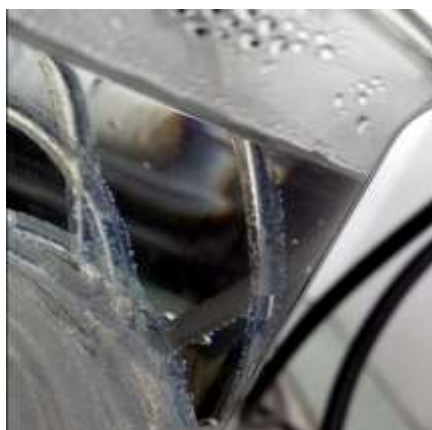
Figure 4-16 unsuccessful polyesterification of succinic acid and propanediol in flow mode using FEP tubing (i.d. = 1.55 mm), where the tube is clogged.
