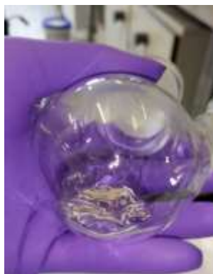
Figure 3-19 PCL obtained instantly after the addition of the monomer to the reaction media in presence of the catalyst t\text{-BuP}_4 and the absence of initiator
