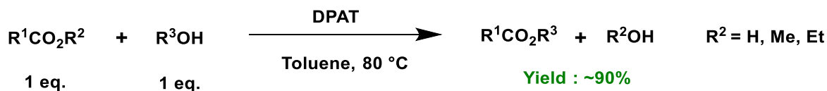
Scheme 4-1 Esterification or transesterification catalyzed by DPAT (adapted) 14
