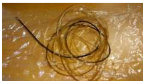
Figure 4-17 Nafion™ tube and its chemical structure
