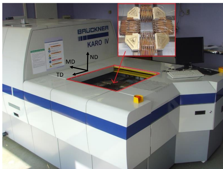
Figure II. 2. A photo of biaxial stretcher with zoom of central film stretching zone.
