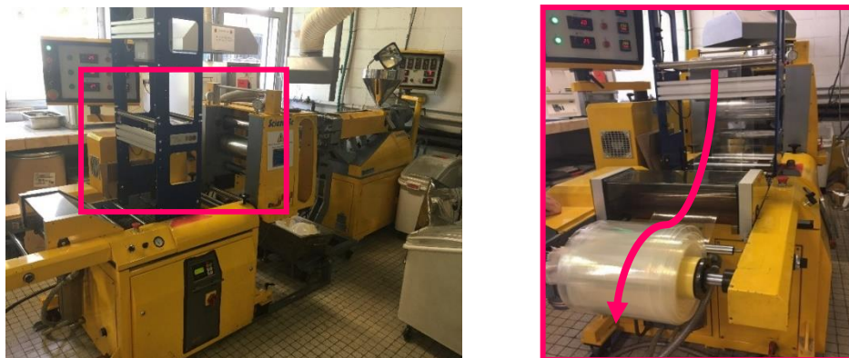
Figure II. 1. Extrusion processing line used for film elaboration.
