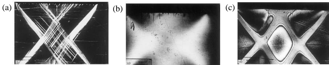
Figure I. 6. Optical microscopy observations of shear bands of various polymers under plain strain compression tests: (a) PS deformed at 20°C (b) PS at deformed 90°C and (c) PC deformed at 20°C (Quinson et al., 1997).
