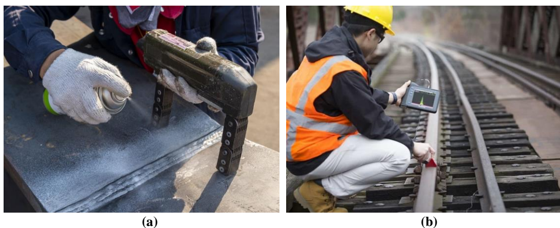
Figure 23: (a) Magnetic particle testing for inspecting a welded piece [54]; and (b) ultrasonic testing involving sound waves for defects detection in rail steels [55]
