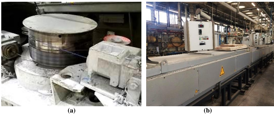
Figure 52: Pilot plants at the Bekaert Technology Center: (a) multi-pass drawing machine and (b) automated heat-treatment line
