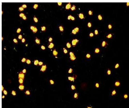
Figure 4.9 B. amyloliquefaciens 98/7 wild type spores appear yellow-orange roundly shaped on stainless steel after staining with Orange Acridine (0.01%).
