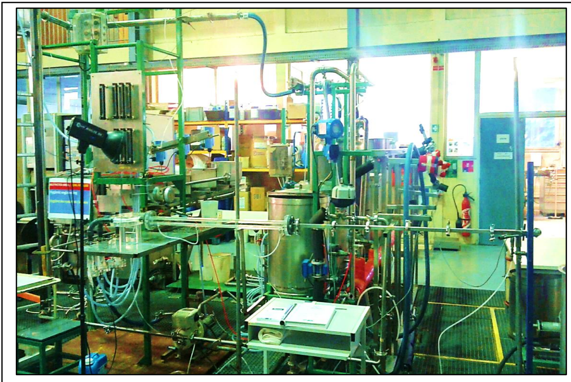
Figure 4.1a. Foam cleaning in place prototype
