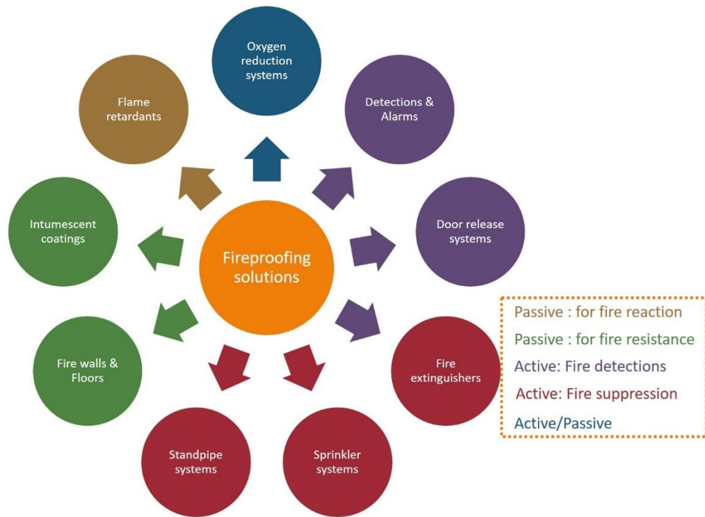
Figure 3. Active and passive fireproofing solutions.
