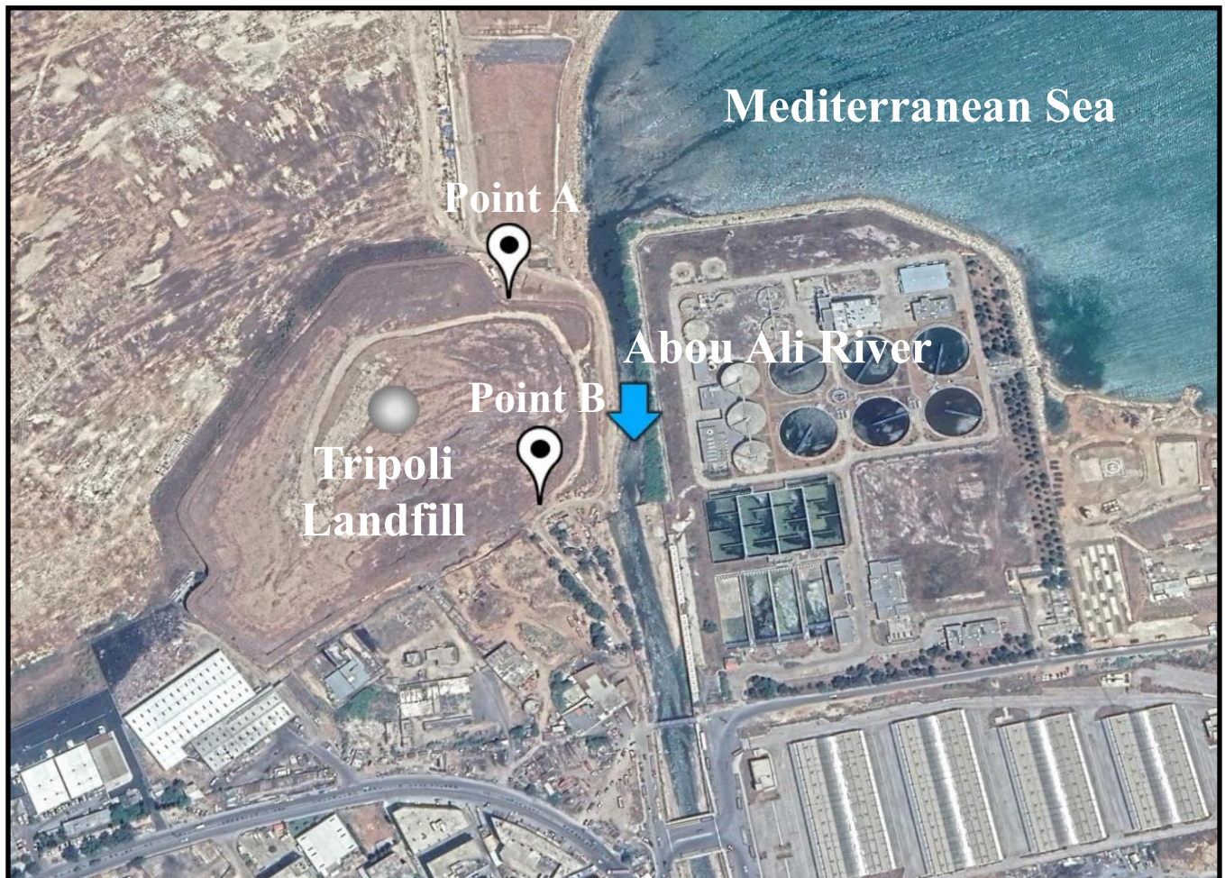
Figure 15: A map showing the location and the sampling points of leachate from Tripoli landfill.
