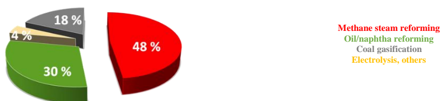
Figure 1: Primary energy distribution through the sources for the production of hydrogen, adapted from ref. 6,7 .
