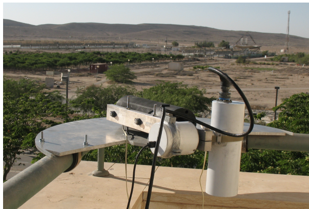
Figure 2.4: CLIMAT measuring set up in the field, where the reference blackbody, the robot arm and the optical head can be appreciated.
