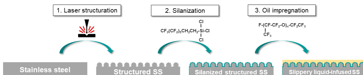
Figure 73. SLIPS-like surfaces process fabrication workflow.
