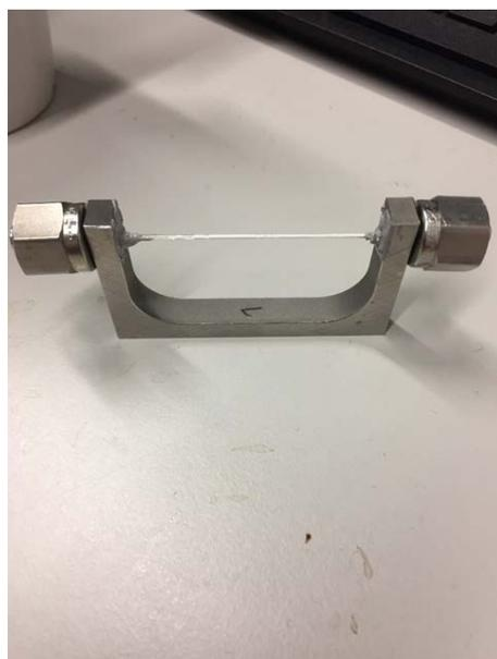
**Figure 3.** Experimental setup used for in-situ XAS measurements.
