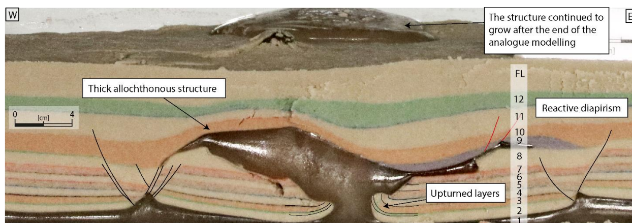
Figure 4.31: Section S02-07, at 17 cm from the southern limit of the box model. We can appreciate the extensional faults both above the autochthonous silicone (black lines) and above the overhang (red lines), these last one result of the gravity spreading and later of the gravity gliding above the salt overhang. The numbers represent the layers deposited on the model (Table 4.2).
