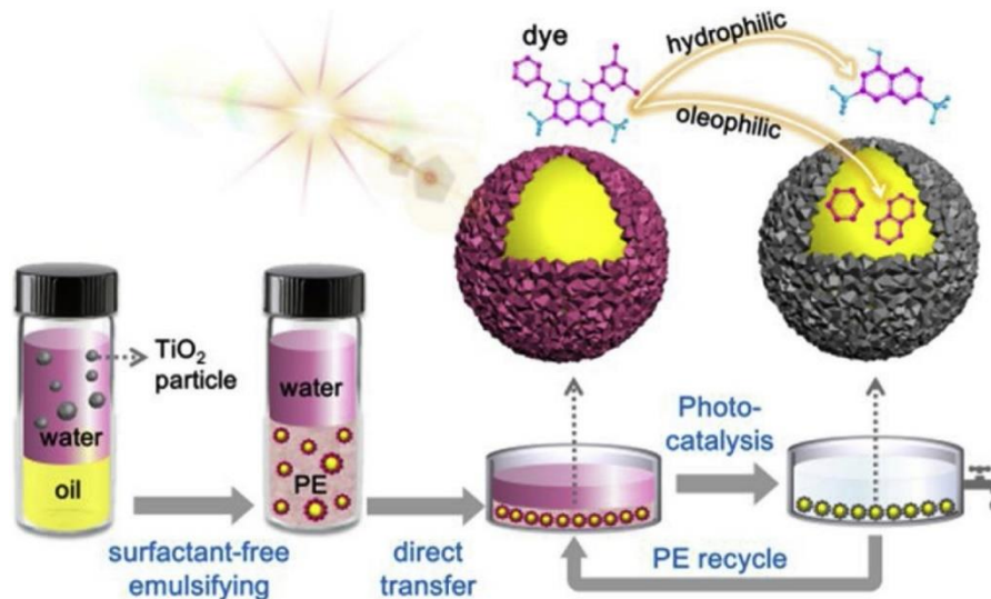
Figure 18. Schematic representation of photocatalytic dye degradation in O/W Pickering emulsion stabilized by commercial \text{TiO}_2 NPs. The dye molecules attached on the surface of \text{TiO}_2 and tuned its wettability to be an emulsifier. (Ref 148 with permission from Elsevier)
