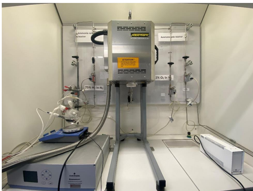
Figure 4. Catalytic set-up for ammonia synthesis and ammonia decomposition developed during this PhD
