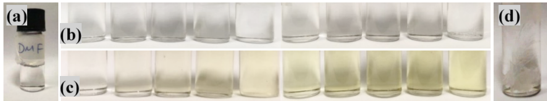
Figure 4.12 a) DMF b) LiBr 1-10w/w% c) KI 1-10w/w% d) 10w/w% LiCl 10w/w% crystal growth [24]
