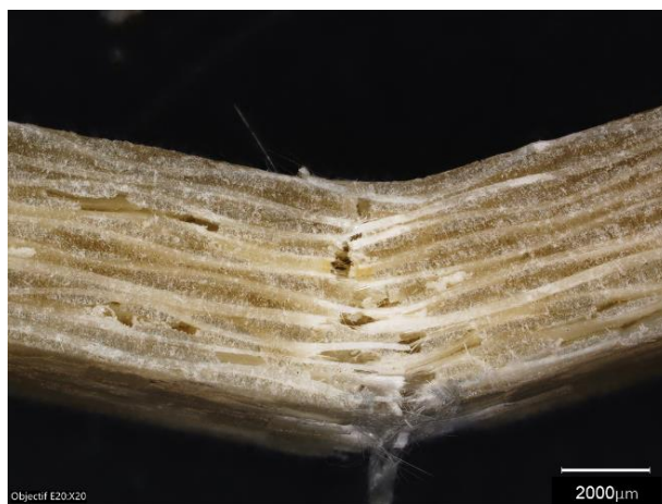
Figure 69: Digital micrograph showing the failure observed in the 10 PLLA/GF specimen.
