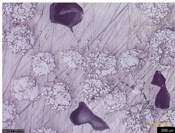
Figure 104: Meso-voids present between flax fiber bundles in a longitudinal cut of PLLA/UD plates.
