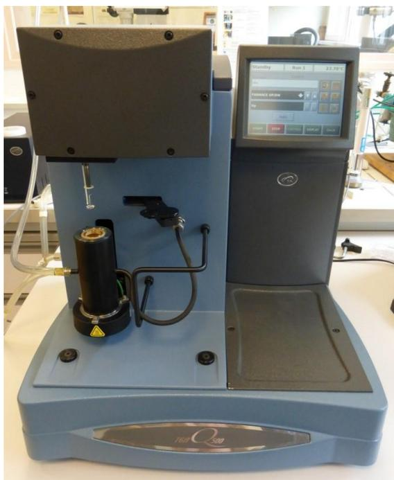
Figure 16 – TGA Q500 (TA instruments, France)
