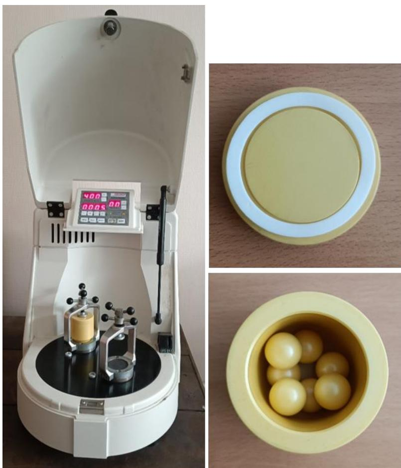
Figure 14– Planetary mill (left) and milling vessel containing seven milling balls (right)
