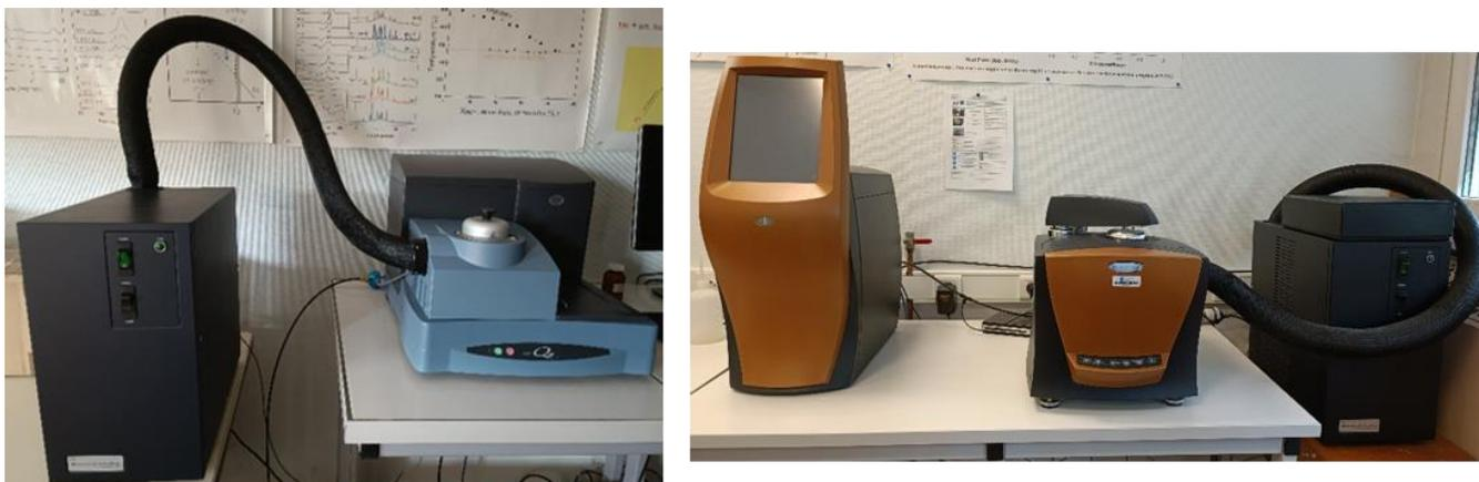
Figure 17 - DSCQ20 (TA instruments, France) on the left-hand side and DSC Discovery (TA instruments, France) on the right-hand side.
