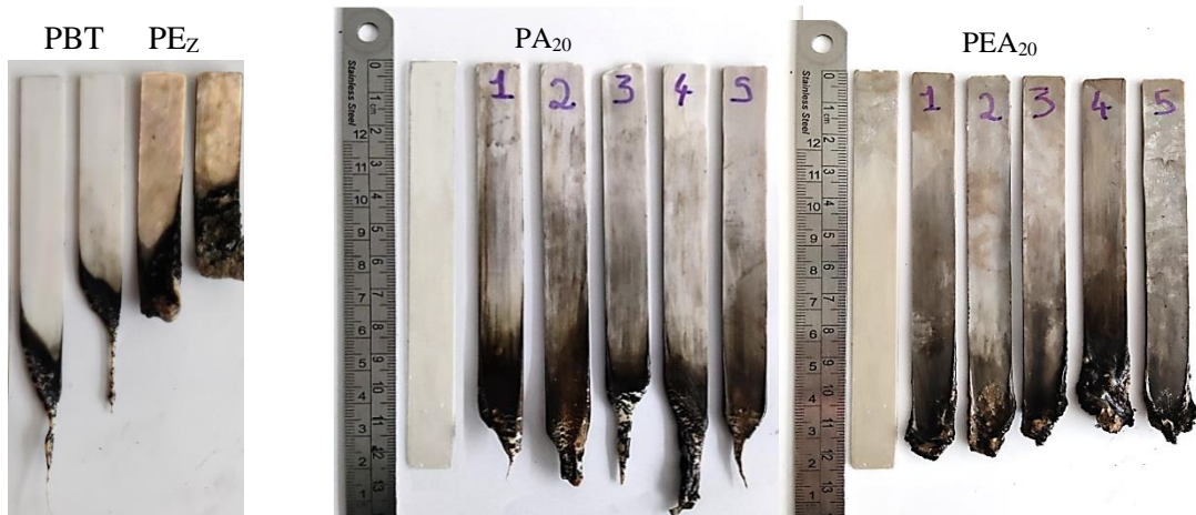
Figure 105 : UL94 samples of PBT and PEZ (combustion stopped to observe the samples) and before and after test for PA 20 and PEA 20 .
