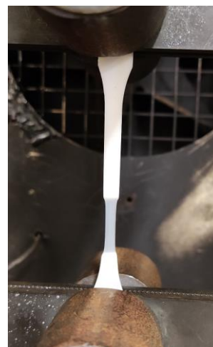
Figure 101 : Left: Stress-strain curve obtained by tensile test at room temperature for PBT and PE z . Right: Picture of PBT dog-bone sample during uniaxial tensile test, exhibiting a heterogeneous deformation.
