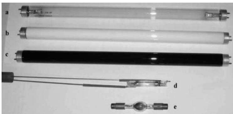
Figure 1-14: Lamps used for photochemical syntheses
