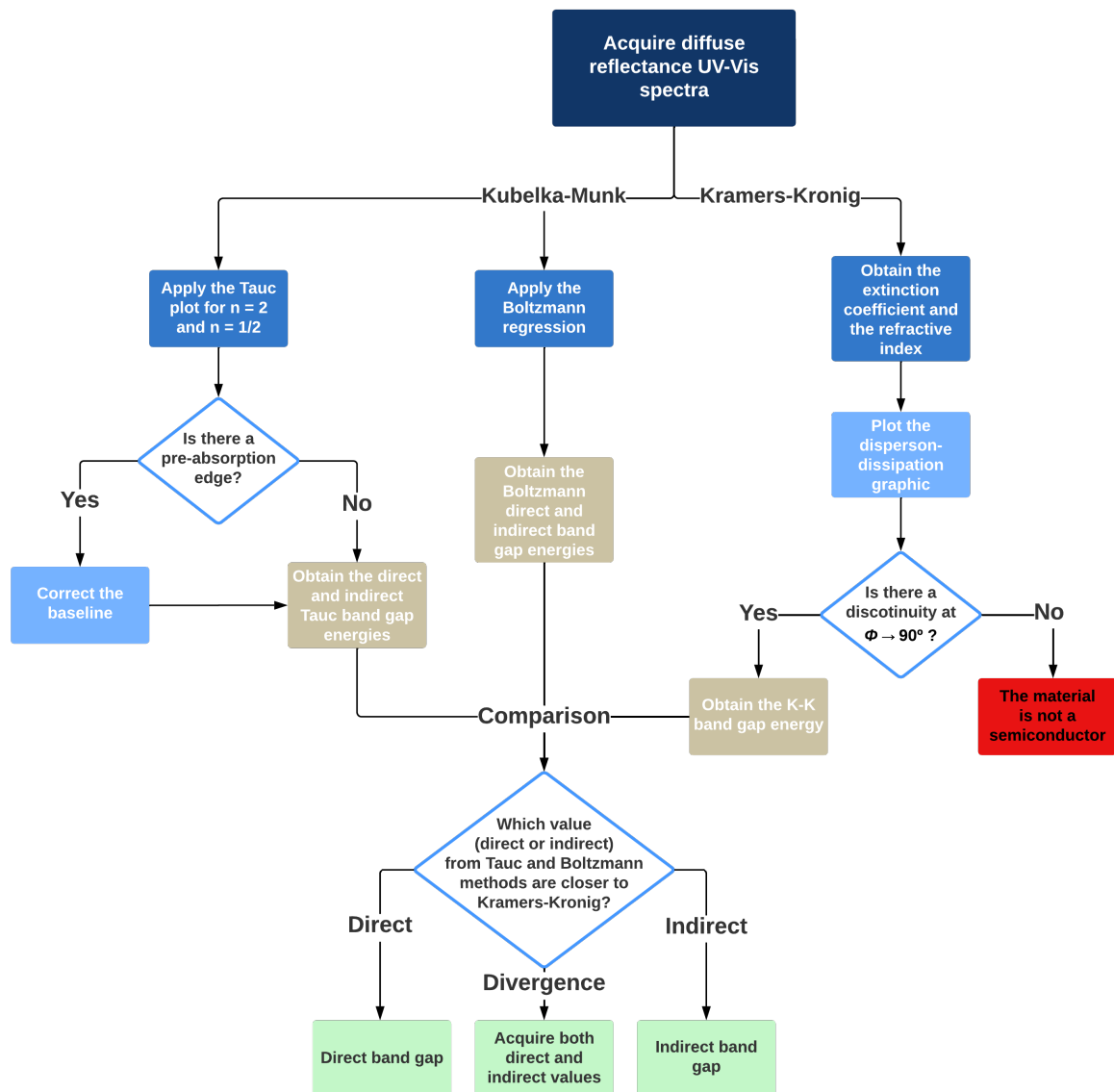
Figure 3.12: Flowchart demonstrating the methodology for determining whether a material has a direct or indirect band gap transition.
