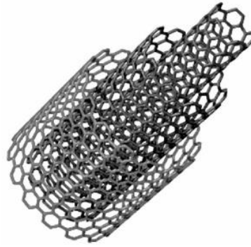
Figure 1.11. Multi-walled carbon nanotubes [44] with Russian doll model.
