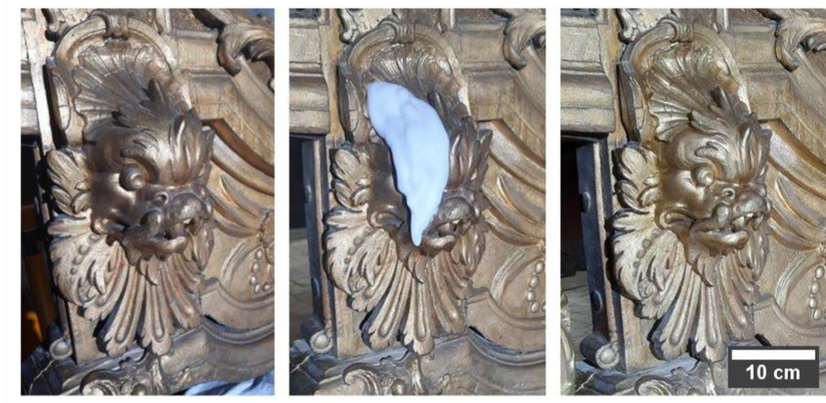
Figure 1.5.4: Historical object (left) before cleaning, (center) during cleaning with foam, and (right) after cleaning The figure was reproduced from (Schad et al., 2022b).
