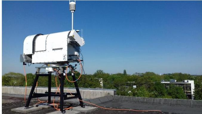
Figure 2.6: Picture of the RPG-HATPRO G5 Radiometer used in this study
