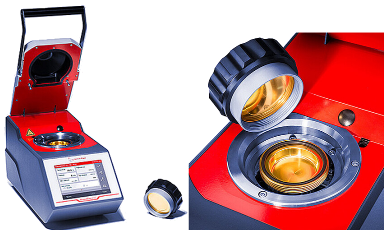
FIGURE 2.7 – RapidOxy 100 Fuel instrument and its gold-plated chamber. Reproduced from anton-paar.com/corp-en/products/details/rapidoxy-100 .
