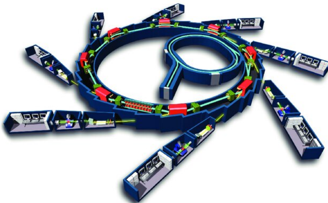
Figure 4.2: Schematic representation of a synchrotron light source. Electrons (blue) are generated by an electron gun and accelerated in a linear accelerator (LINAC) before being injected into a storage ring. Bending magnets (red) alter the electron trajectory, causing the emission of synchrotron radiation (yellow), which is directed toward experimental stations [5].
