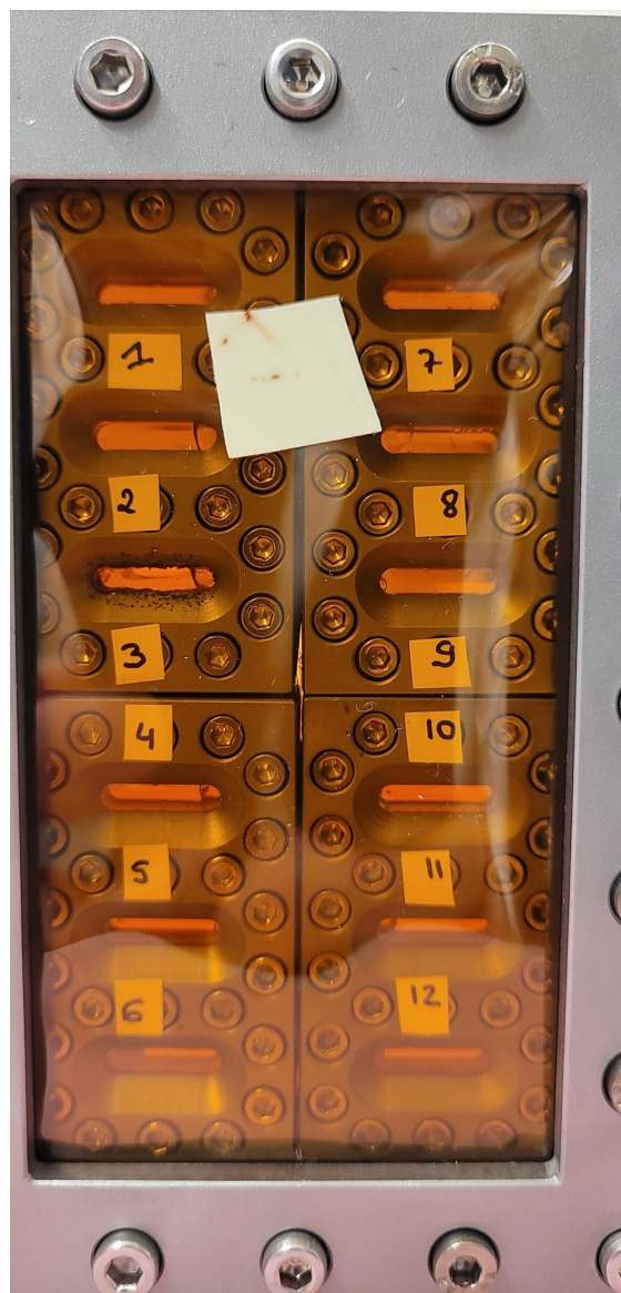
Figure 4.1: EXAFS cells containing protactinium samples prepared at IJCLab (Orsay) for measurements at the MARS beamline of the SOLEIL synchrotron. The sample numbering corresponds to Table 4.1. The analyses were performed at the Pa L_3 -edge during an experimental campaign conducted from February 14 th to 19 th , 2024.
