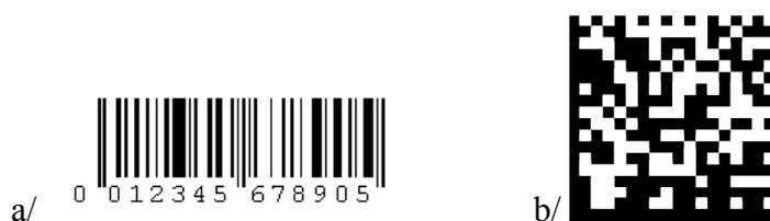
*Figure 2.1 : a/ EAN13 - b/ Datamatrix*
