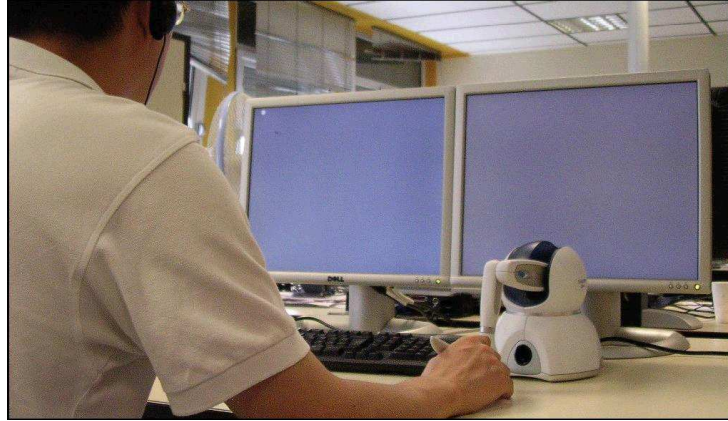
Figure 2.6: Experimental Apparatus: Simulating the RubberEdge hybrid technique and position control with a PHANToM haptic device
