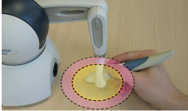
Figure 2.5: Simulating the RubberEdge hybrid technique with the PHANTOM haptic device. A 2D simulated haptic surface constrains the pen movement and the elastic zone is created using force feedback.
