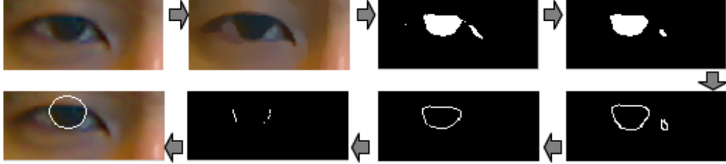
Figure 6.9: Illustration of iris ellipse fitting. Follow the arrow direction: Original eye image \rightarrow MeanShift Segmentation \rightarrow Histogram-based binary segmentation \rightarrow 'Open' morphology \rightarrow Canny edge operation \rightarrow Largest contour finding \rightarrow Keeping near vertical edge points \rightarrow Fitted ellipse
