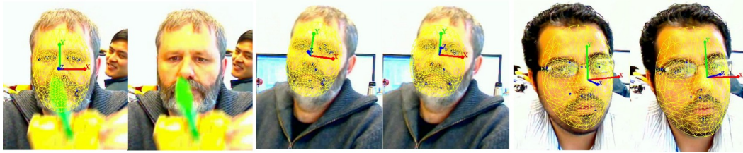
Figure 4.8: Comparing the tracking performances of single-view with multi-view class detection. The left image of each pair is the single-view based performances. Both tracking inaccuracy and failures are reduced due to the fact that more class views lead to more matches.
