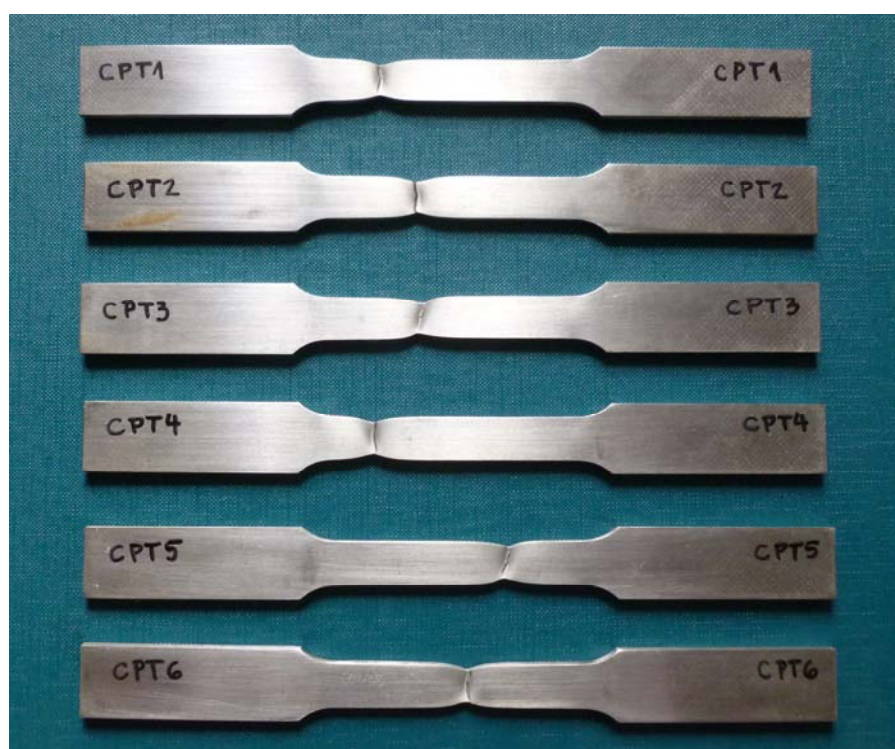
Figure III.7. Tension test coupons after rupture.
