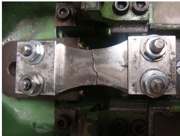
Figure IV.1. Fatigue test sample after rupture.
