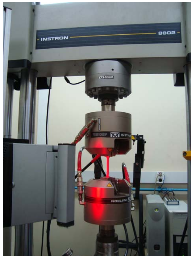
Figure III.5. Setup for uniaxial tension tests with a conventional servo-hydraulic machine (Instron 8802) and a video extensometer.
