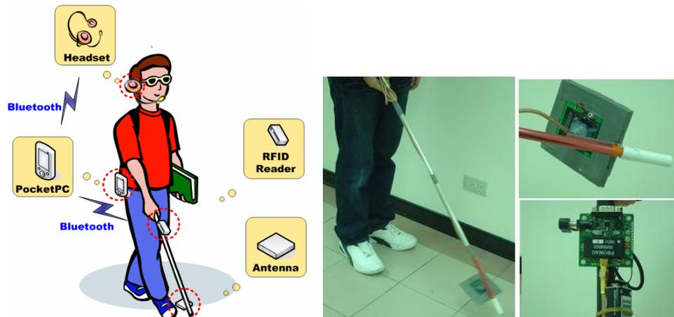
Fig. 1.10: On the left hand side of the figure is the *iCane* overview; on the top right of the figure is RFID antenna; on the bottom right of the figure is RFID reader [28]
