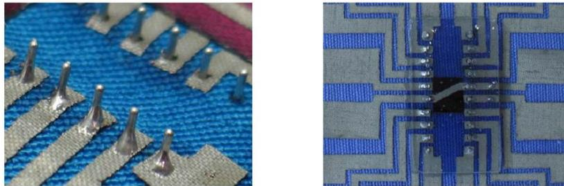
Fig. 1.47: Solder joints on a fabric PCB [146]
