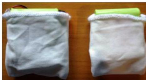
Fig. 4.56: Removable fabrics for microcontroller and pockets for batteries
