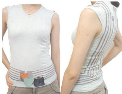
Fig. 1.54: Prototype of garment with electrical nerve stimulation (TENS) function [183]
