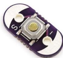
Fig. 4.46: Arduino LilyPad Button Board® [290]
