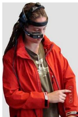
*Fig. 1.52: A virtual 3D mobile guidance jacket [173]*
