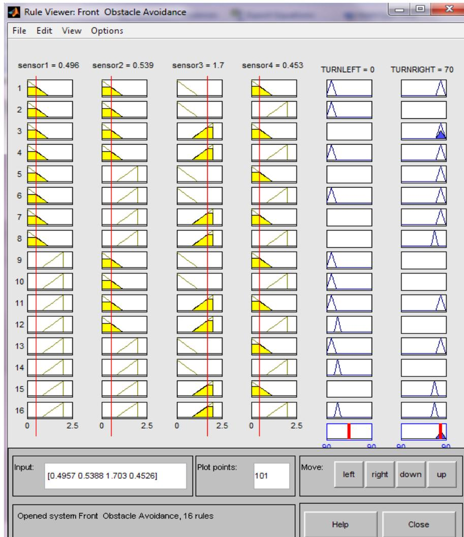
Fig. 4.27: Implication and defuzzification process of front obstacle avoidance neuron fuzzy inference
