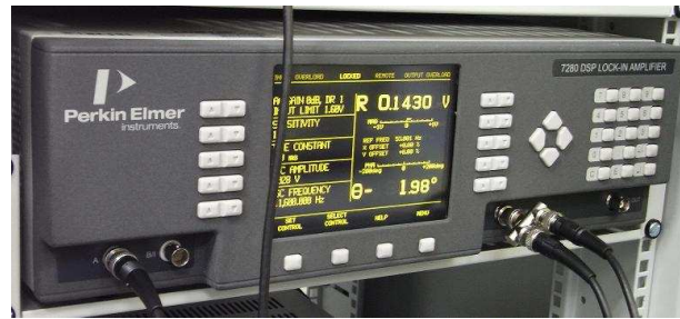
Figure 7.5: Signal Recovery 7280 DSP Lock-in Amplifier.
