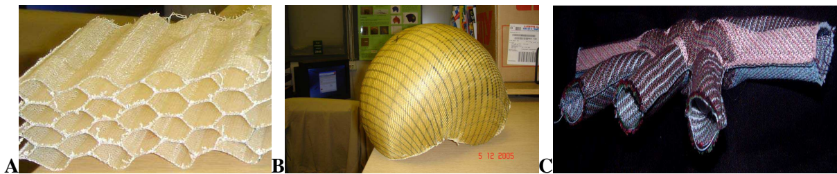
Fig. 1.1: 3D Profiled fabrics (A) Hollow (B) Shell and (C) Nodal Type [5]
